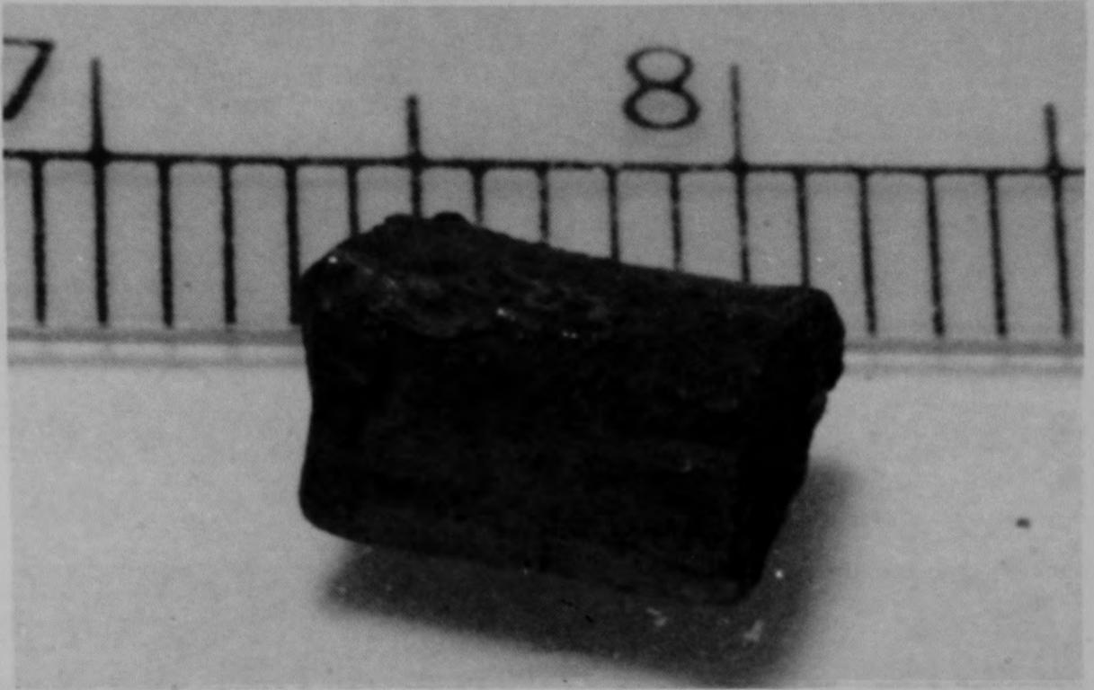
Figure 12. Photograph of Particle 1B (H8, surface) showing an example of a fuel piece.
